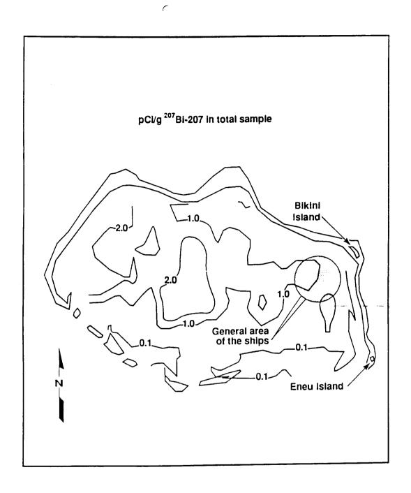
Figure 3. Bismuth-207 Concentration contours in the lagoon surface sediments at Bikini Atoll in 1979.
