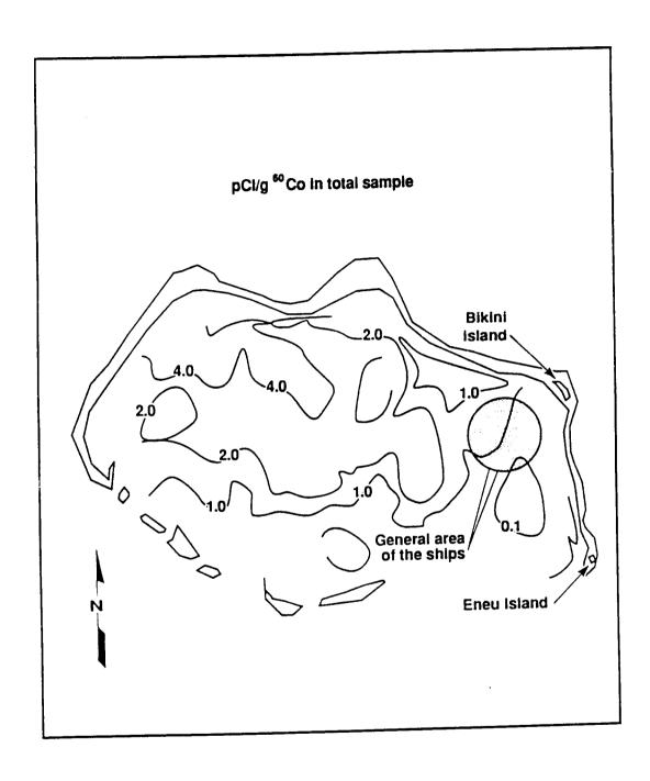
Figure 2. Cobalt-60 concentration contours in the lagoon surface sediments at Bikini Atoll in 1979.
