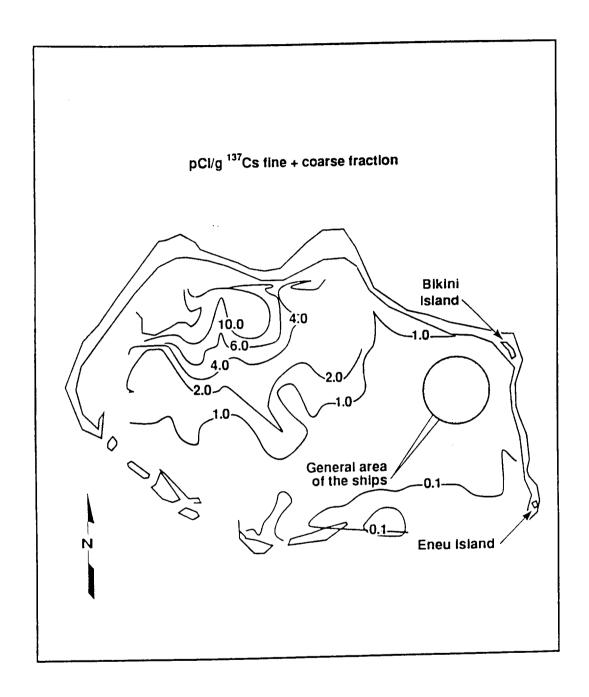
Figure 1. Cesium-137 concentration contours in the lagoon surface sediments at Bikini Atoll in 1979.
